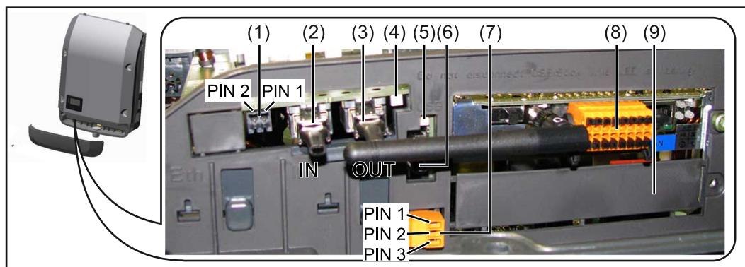
Depending on the model, the inverter may be equipped with the Fronius Datamanager plug-in card (8).
