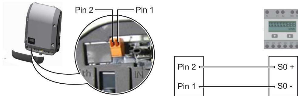
The SO meter must comply with the IEC62053-31 Class B standard
