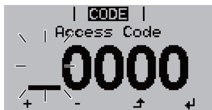
"Access Code" is displayed in the "CODE" menu; the first digit starts flashing.
