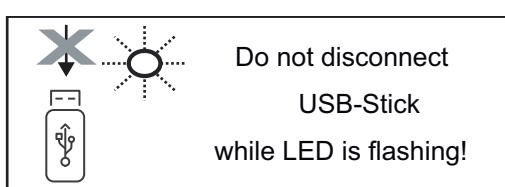
**IMPORTANT!** To avoid any loss of data, a USB flash drive may only be removed if the following conditions are met:
