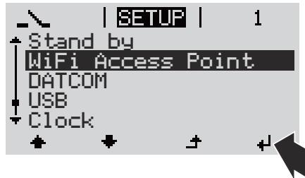
The inverter establishes the WLAN access point. The WLAN access point remains open for 1 hour. The protection switch on the Fronius Datamanager 2.0 can remain in switch position A due to the activation of the WLAN Access Point.
