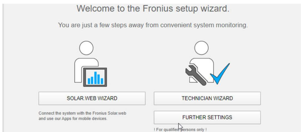
The technician wizard is intended for the installer and contains standard-specific settings. Running the technician wizard is optional.
